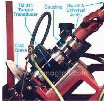
A Model TM 311 Torque Transducer is used in the design along with a disc brake, coupling, swivel and universal joint for accuracy and reliability.
