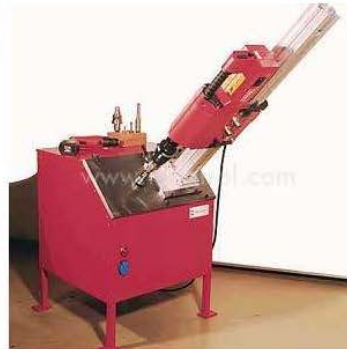
BRP 125 Test Bench specially designed for testing torque limiter on a wide range of drills from 5 Nm to 200 Nm.
